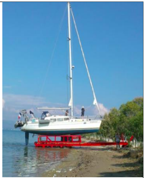
Lift out by tractor and trailer
